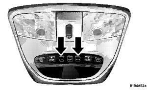
2. Position the end of your hand-held transmitter 1-3 inches (3-8 cm) away from the HomeLink buttons while keeping the EVIC display in view.
